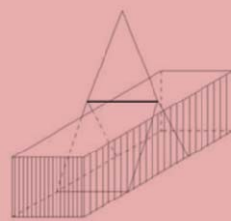
(b) With spreader beam, lift points at lower module floor
